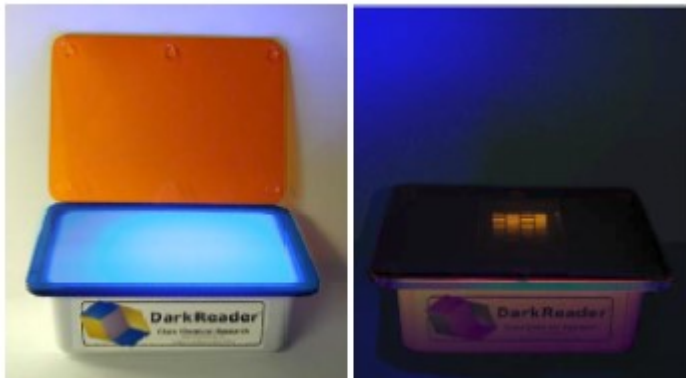
A DR45M transilluminator is shown above 'at rest' and viewing a SYBR Gold-stained DNA gel.
