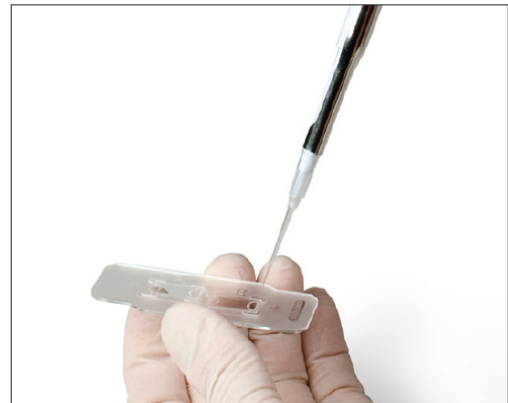
Fig. 9. Loading the counting slide.
